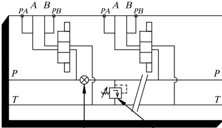
Tapped hole 3/8"G for possible plug to separate the P of first station (plug out of supply)
