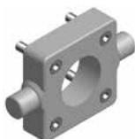
Intended for articulated mounting of cylinder. This trunnion can be flange mounted on the front or rear end cover of all P1D cylinders.
