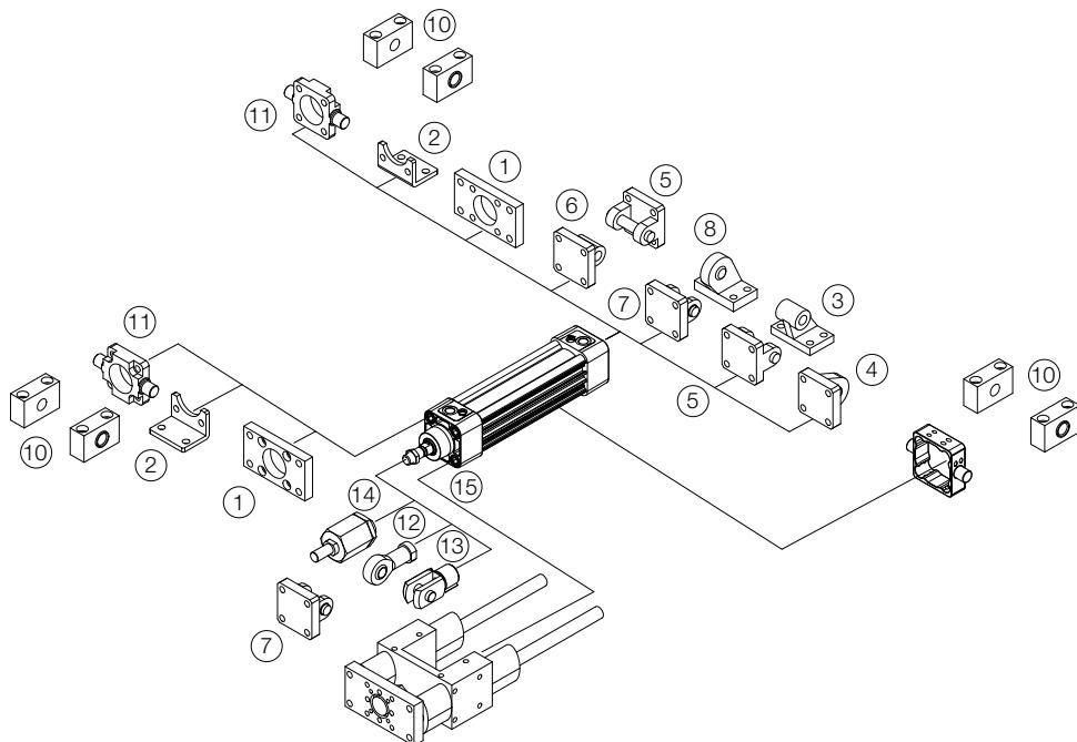
**P1D-B Pneumatic ISO Cylinders****Cylinder mountings****Flange MF1/MF2 ①**
