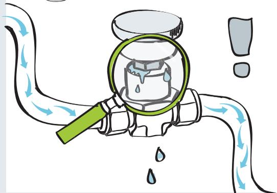
**#5** Tighten the packing nut
