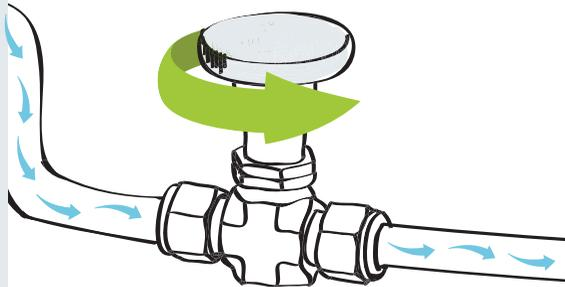
**#3** Detect for stem leakage
